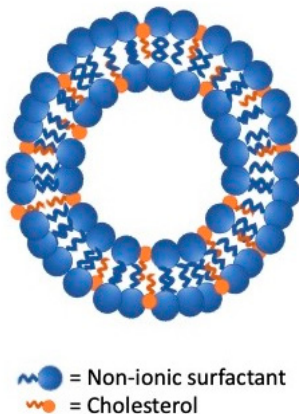
Figure 1. Structure of proniosomes lipid vesicular systems.
