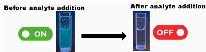
Figure 4. Fluorescence quenching of blue emitting BCCDs in the presence of Fe(III) ions reported in [85]. Reprinted with permission from Elsevier.
