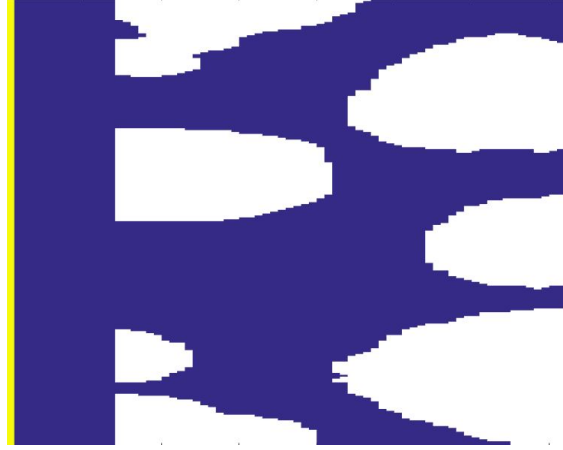
Figure 4.10: Example of simulation initialization with \rho = 0 (blue) everywhere except that at the inlet cells where a constant \rho > 0 (yellow) is imposed. In this picture the solid grains are represented in white.
