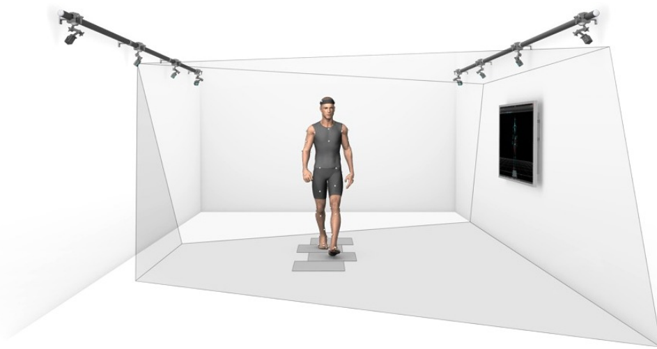
Fig. 1.7 Schematic of motion capture systems including markers positioned on the subject's body and cameras (from [107]).
