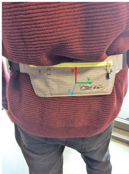
Fig. 3.10 Smartphone position adopted for the experiments.
