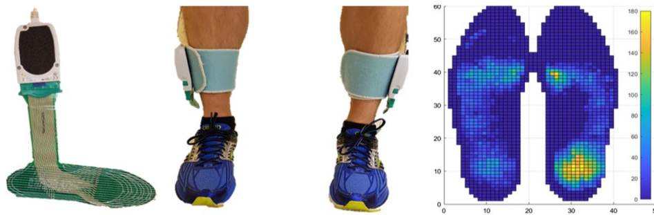
Fig. 1.9 Smart pressure insoles system, positioning, and generated foot pressure map (from [124]).
