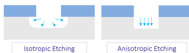
Figure 7. The isotropic and anisotropic behavior of wet- and dry-etching.
