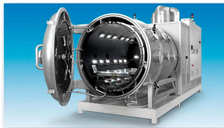
Figure 6. The thermo-vacuum chamber employed in the tests.
