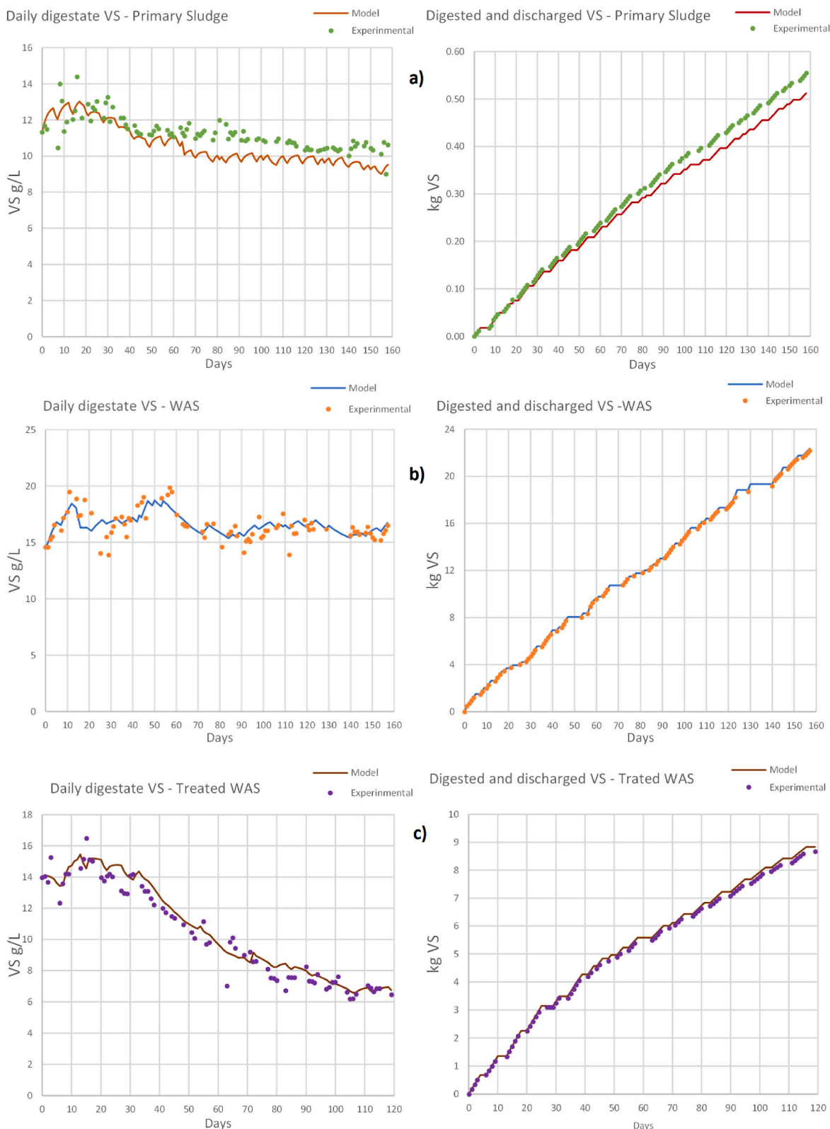
Fig. 6. Daily digestate VS concentrations and cumulative discharged VS during the semi-continuous AD tests involving the PS (a, test n.1), raw WAS (b, tests n.2) and treated WAS (c, tests n.3).
