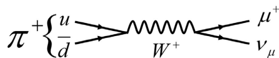
Figure 5 – Lowest order Feynman diagram showing the decay of the \pi^+ - meson into muons and neutrinos via a W^+ boson. The decay for the \pi^- - meson is similar, only with opposite charge conservation.
