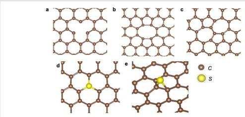
Figure 4. Detail of optimised models illustrating typical hard carbon defects (a) MC, (b) divacancy, (c) Stone-Wales rotation; and (d) and (e) the two common sulfur-carbon bonding considered in this work.
