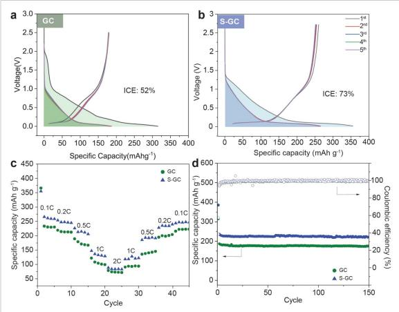
**Figure 2.** Galvanostatic charge—discharge profiles of the first five cycles for: (a) pristine hard carbon (GC) and (b) sulfur doped hard carbon (S-GC). (c) Specific capacity and Coulombic efficiency of GC (green circles) and S-GC (blue triangles) during 150 charge—discharge cycles; (d) Specific capacity for GC (green circles) and S-GC (blue triangles) under varying C rates (from 0.1 C or 30 mAg<sup>-1</sup> up to 2 C or 600 mAg<sup>-1</sup>).
