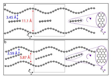
**Figure 3.** Optimised geometries of the final pore (a) and graphitic (b) models. The initial building unit is shown in the centre highlighted by a square and their periodic images are shown in both sides for the sake of facilitating visualisation. On the right side we show a rotated view of the sandwiched graphene ribbon which is continuously periodic in *y*-direction and periodically repeated in *x*-direction.
