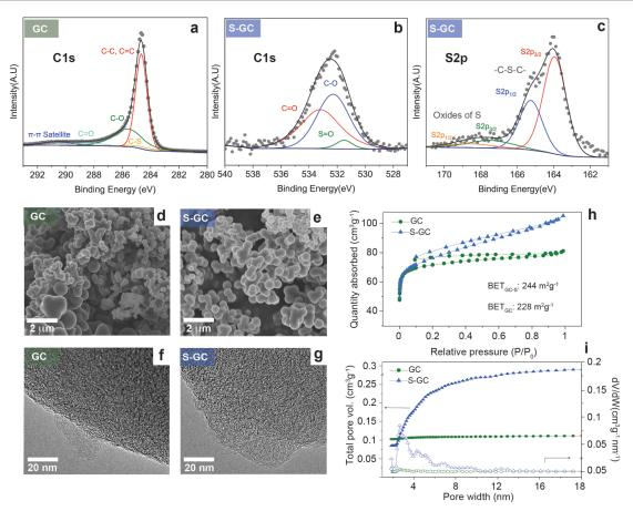
**Figure 1.** High resolution C1s XPS spectra for: (a) pristine hard carbon (GC) and (b) sulfur doped hard carbon (S-GC). (c) S2p spectra for S-GC. SEM and TEM images of GC (d) and (f) and S-GC (e) and (g) showing no evidence of microstructural changes upon doping. Nitrogen adsorption isotherms (h) and Cumulative pore volume (i) for both materials.
