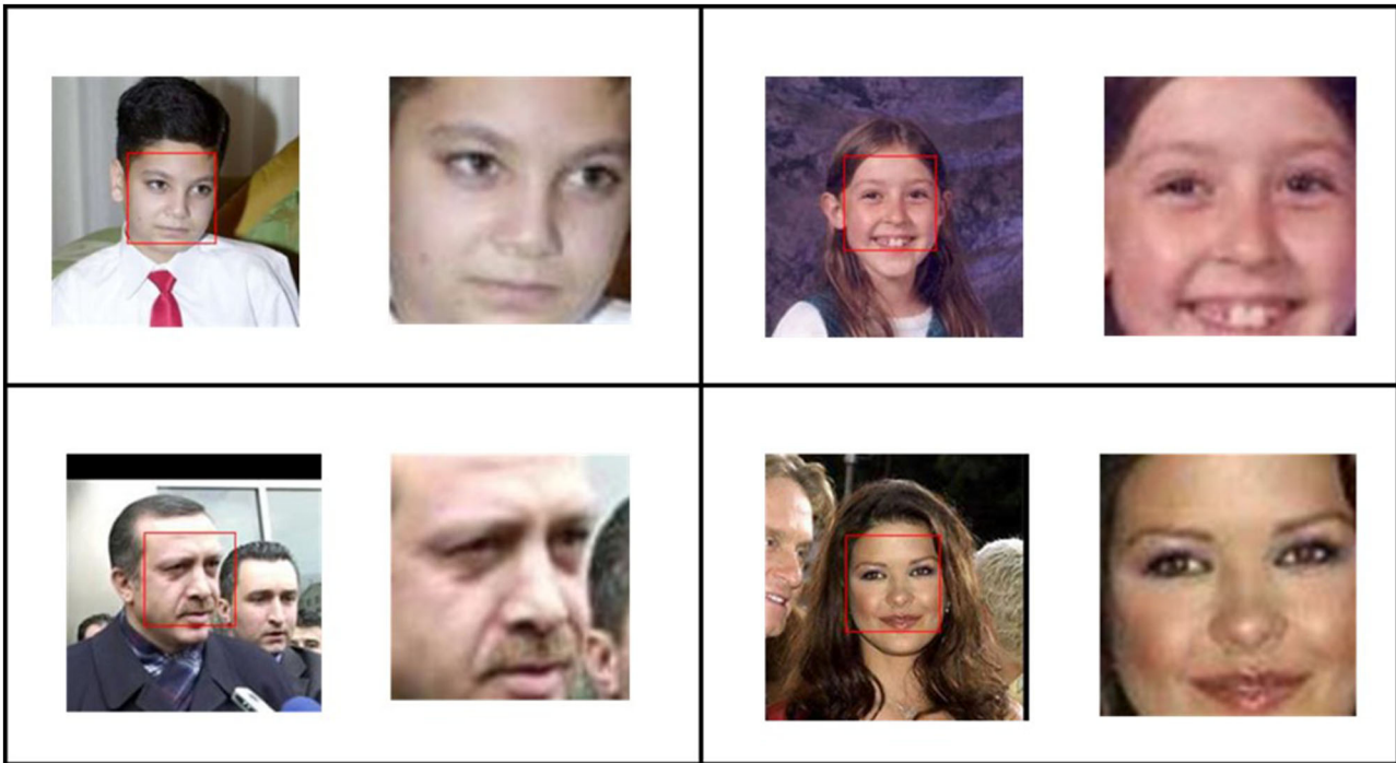
FIGURE 1 Face region selection using an oriented gradient-based algorithm (Dalal and Triggs, 2005) on AFW dataset faces; left image in each cell is original where red box is representing the detected face and right one is the automatically cropped face region.
