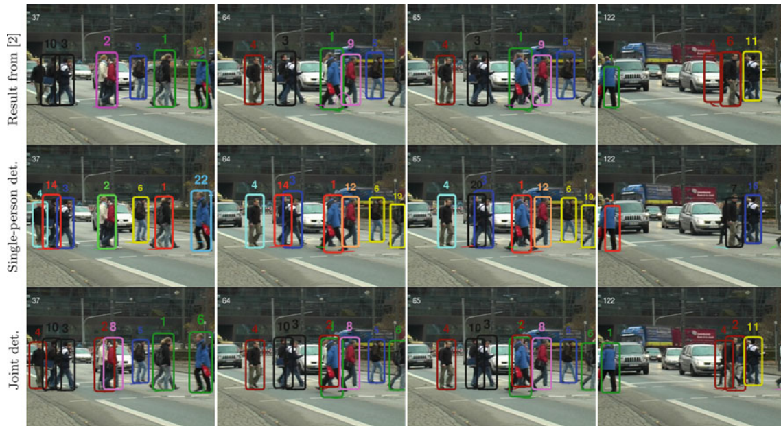
Fig. 11 Tracking results on the TUD-Crossing dataset obtained with the approach of Andriyenko and Schindler (2011) (top row), our single-person detector (middle row) and our joint detector (bottom row). Colors and numbers indicate tracks corresponding to different people
