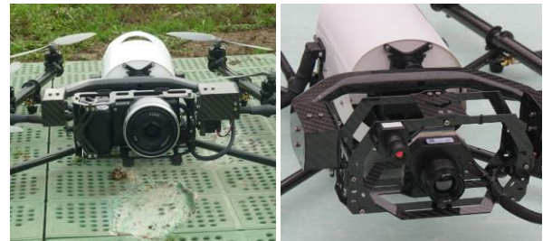
Fig. 6. Cameras (RGB and TIR) mounted on the Falcon that were used for this survey.
