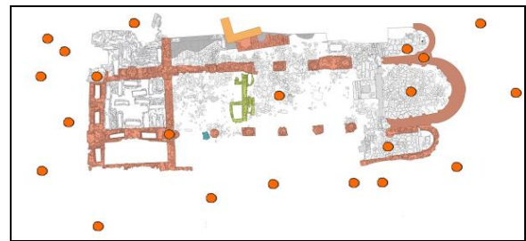
Fig. 5. Scan positions for the laser survey.
