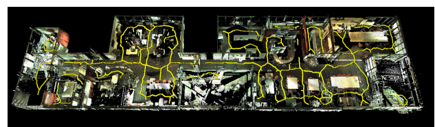
Figure 10. Geometrical network model overlaid into point clouds
