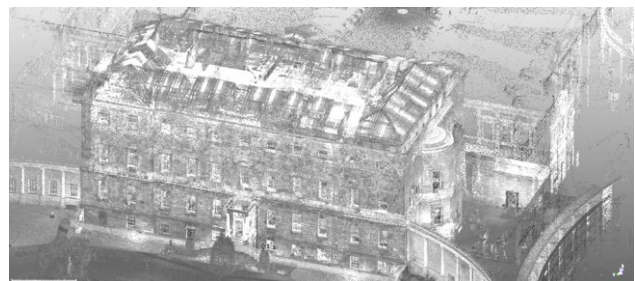
Figure 5: Point Cloud from Time of Flight Scanner
