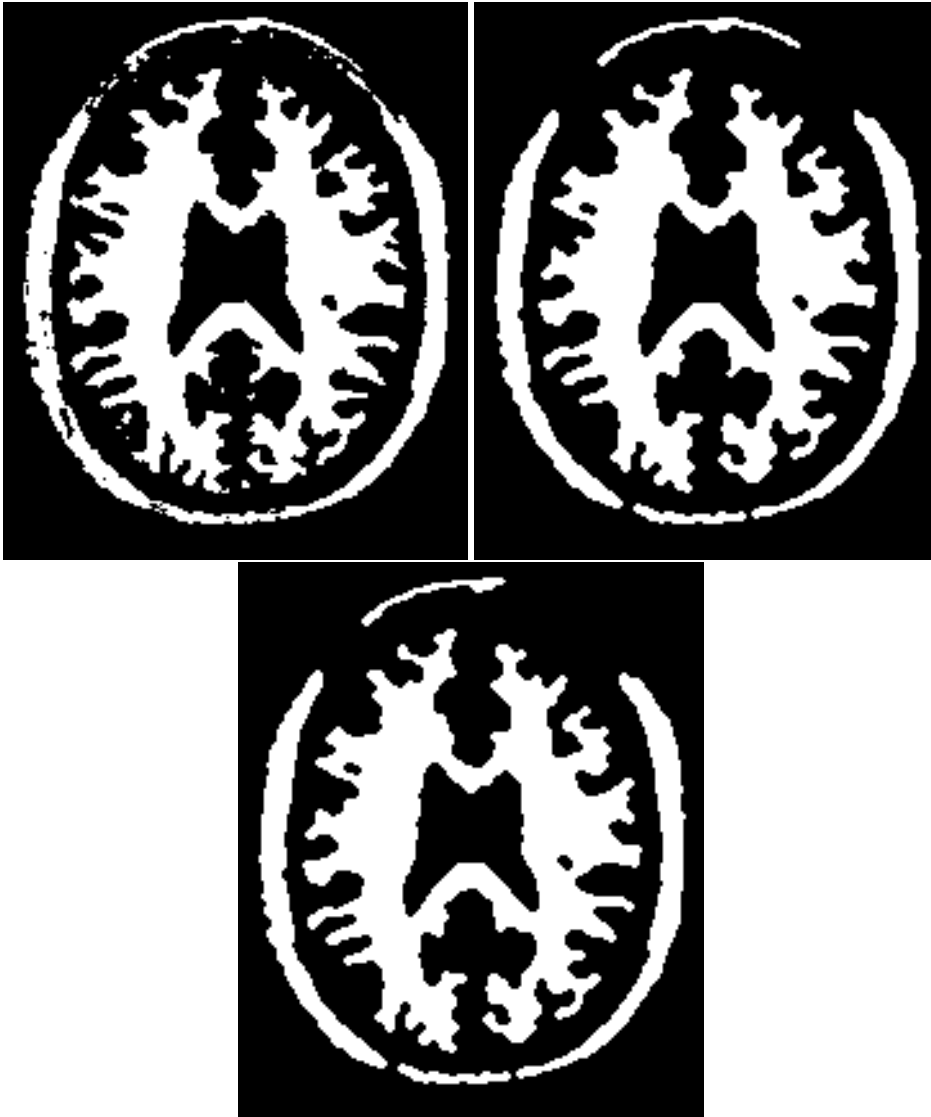
Figure 2.17: Effect of 1, 10 and 50 iterations of the BinaryMedianImageFilter using a 3x3 window.
