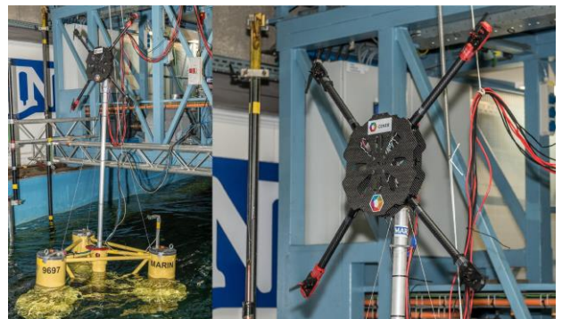
Figure 194: MARINET2 tests with CENER's multi-fan actuator system tested at MARIN (courtesy of CENER).
