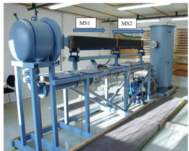
Figure 39: Friction tunnel (Schulze & Klose, 2017)
