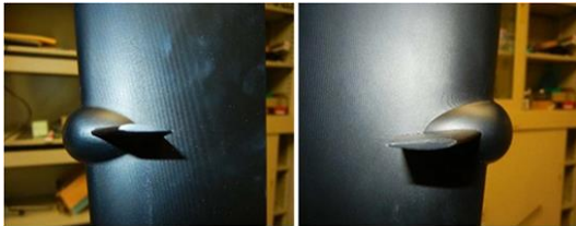
Figure 33: Rudder bulbous fin system (Truong et al., 2017)
