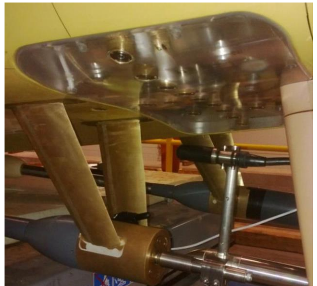
Figure 66. Flush-mounted transducer set up used by Foeth & Bosschers (2016).
