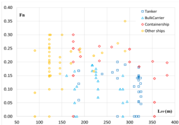
Figure 120 Main features of the ships, and the tested Froude numbers and the wave headings in the added resistance database.
