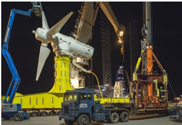
Figure 177: AR1500 tidal turbine test fitting on the dock. (SIMEC ATLANTIS ENERGY, 2019).
