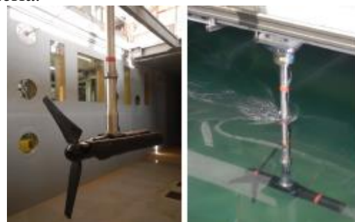
Figure 171: Three-bladed “round-robin” horizontal instrumented turbine in water flume and tow tank (From Gaurier et al. (2015))
