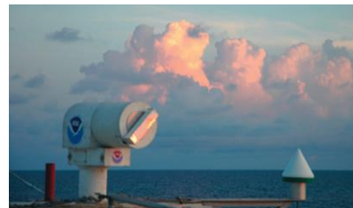
Figure 169 Doppler LIDAR scanner on a vessel [Pichugina, 2012]
