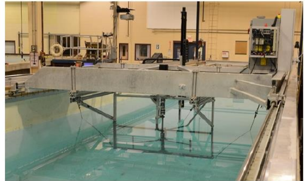
Figure 174: A 1:6 scale cross-flow turbine (DOE-RM2) setup up in tow tank (from Wosnik et al. (2015))
