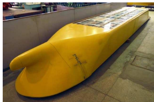
Figure 36: Photo of tanker model with recess (Borusevich et al., 2016)
