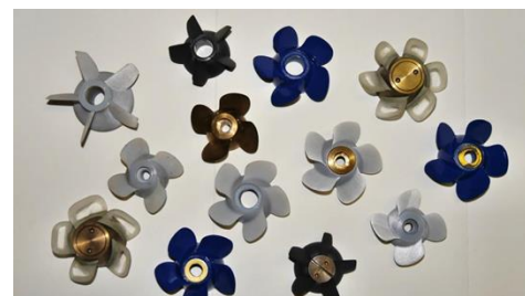
Figure 32: Various hub caps with fins (Müller et al., 2017)
