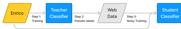
Figure 7: We applied semi-supervised learning to boost screen classification performance using unlabeled web data. First, a teacher classifier is trained using a “gold” dataset of labeled mobile screens. Then, the teacher classifier is used to generate a “silver” dataset of pseudo-labels by running it on a large, unlabeled data source (e.g., web data). Finally, the “gold” and “silver” datasets are combined when training a student classifier, which is larger and regularized with noise to improve generalization. This process can be repeated; however, we only perform one iteration.
