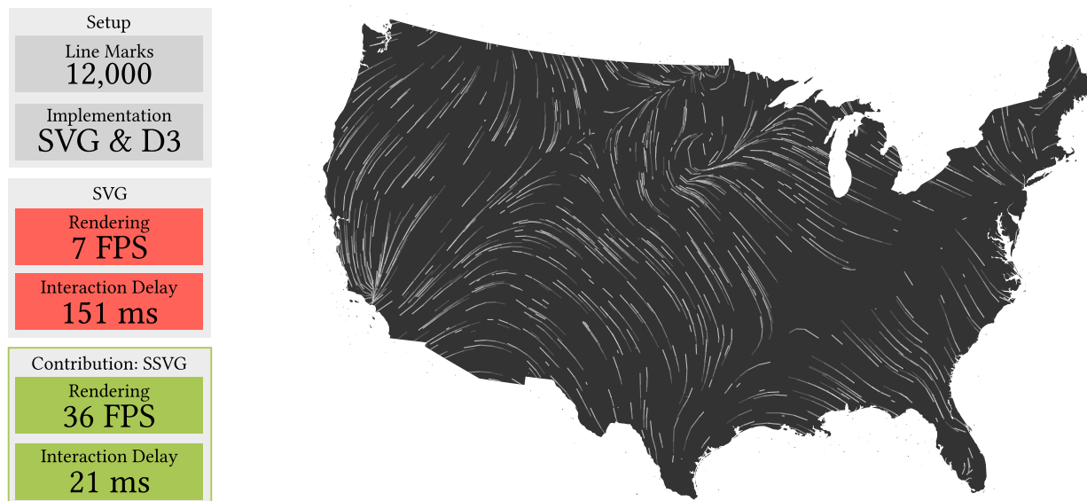
Fig. 1. Viegas & Wattenberg’s popular wind map visualization is written for the Web using Canvas for its rendering speed ( http://hint.fm/wind/ ). Implementation via the more-familiar SVG and D3.js is comparatively simple and enables element-level events for interaction, styling with CSS, and element inspection, but results in slow rendering at 7 frames per second (FPS). Using SSVG, via one line of additional code, we reach 36 FPS. This is faster than the original Canvas implementation. Live at ssvg.io/examples/windmap .
