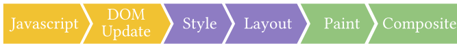
Fig. 3. Chrome’s rendering pipeline performs these steps on the main thread at its tick rate after any JavaScript code updates the DOM: Style, Layout, Paint and Composite. In some cases, these steps take just as much time as the visualization’s JavaScript code itself even though that work is often unnecessary for visualization, such as re-applying CSS rules when styles have not changed or positioning and layering HTML elements even though SVG does not support these features. SVGs are much simpler to render than HTML, yet browser rendering does not take advantage of their simplicity. Figure adopted from [17].
