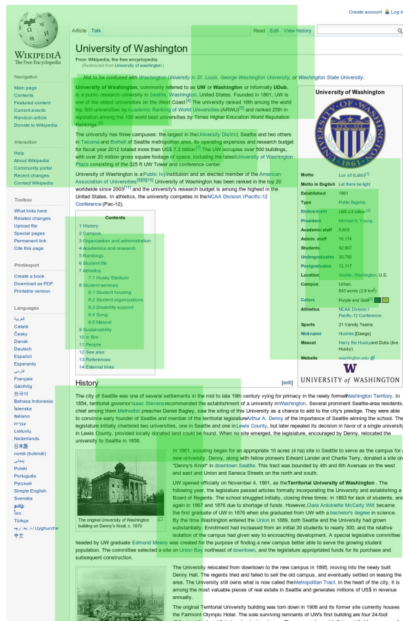
Figure 2. An illustrative example of a heatmap on a Web page generated from mobile device users' viewport data.
