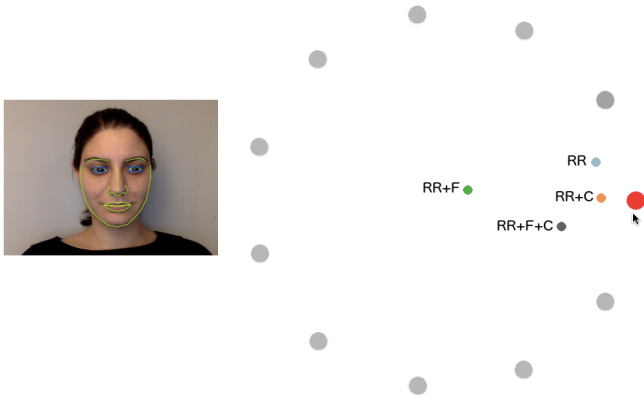
Figure 1: Composite image demonstrating the experimental setup for the target selection task. Clmtrackr is used for facial feature detection. Predictions from different regression models are depicted with different colors. Users aim at the red target.
