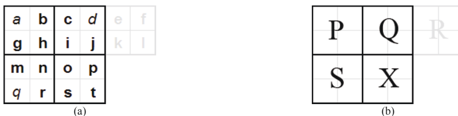
Figure 4 The proposed block-based scan mask or B-Mask (do not check on position R).
