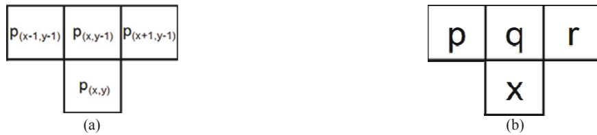
Figure 9 Pixel-based scan mask proposed by He et al. [8]. (a) Pixels coordinate; (b) identifiers of the single pixels.
