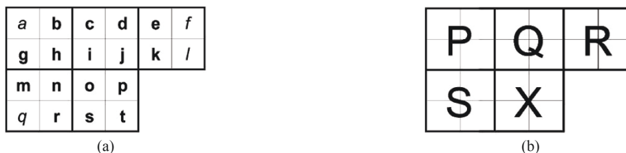
Figure 2 Block-based scan mask [3]. (a) Identifiers of the single pixels; (b) blocks identifiers.
