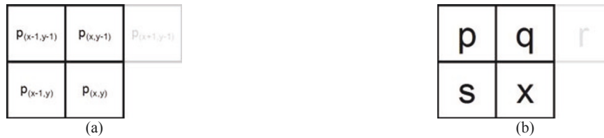
Figure 3 The proposed pixel-based scan mask or P-Mask (do not check on position r).
