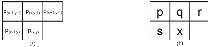
Figure 1 Pixel-based scan mask [5]. (a) Pixels coordinate; (b) identifiers of the single pixels.
