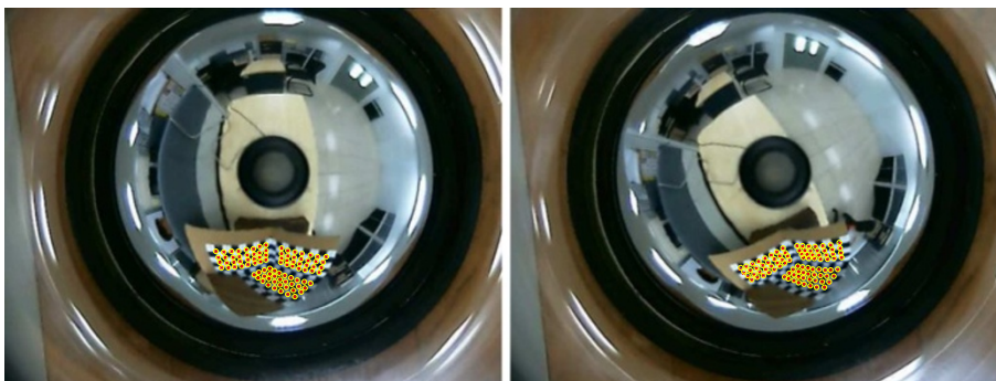
Figure 17 Reprojection of the 3D reconstruction. The reconstructed 3D points are reprojected back to the input images.
