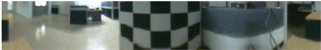
Figure 10 Cylindrical panoramic unwrapping. Common cylindrical unwrapping can be done using an open-ended cylindrical virtual plane.
