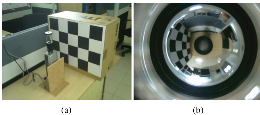
Figure 9 Experiment set-up for panoramic unwrapping. A controlled environment for panoramic unwrapping is set up as in (a) and corresponding omnidirectional view image is captured as shown in (b).
