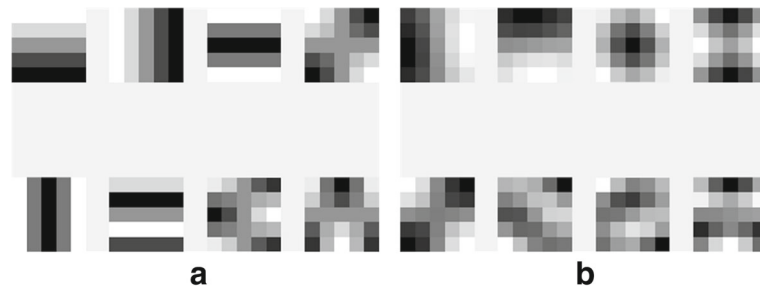
Fig. 2 ICANet filter: The figure shows the filters learned in the ICANet volume base, with the filter size and filter number for both phases set to 11 \times 11 and 8, where a and b are the first and second stages, respectively, of the filter in the ICANet convolutional layer
