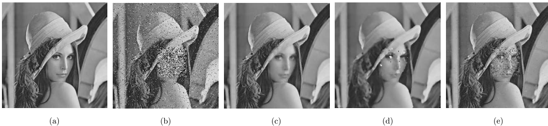
Figure 8: (a) Original image, (b) Corrupted image, (c) Recovered image by Gaussian BP, (d) Recovered image by median filter ( 5 \times 5 ) for all pixels, (e) Recovered image by median filter ( 5 \times 5 ) only for pixels with values 0 or 255.
