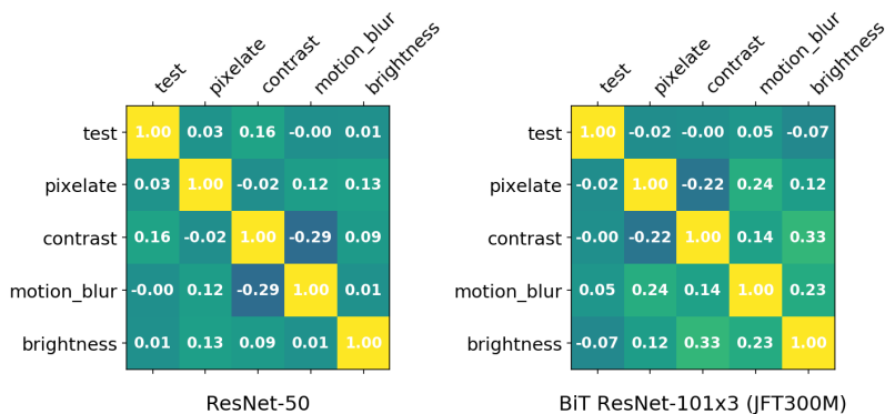
Figure 5: Performance on ImageNet-C stress tests is unpredictable from standard test performance. Spearman rank correlations of predictor performance, calculated from random initialization predictor ensembles. (Left) Correlations from 50 retrainings of a ResNet-50 model on ImageNet. (Right) Correlations from 30 ImageNet fine-tunings of a ResNet-101x3 model pre-trained on the JFT300M dataset.
