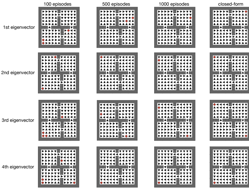
Figure 27: First four eigenoptions discovered online for a varied number of episodes, computed from the eigenvectors in Figure 26. We plot only one eigenoption per eigenvector (instead of two). Policies were learned off-policy from the data collected when learning the SR.
