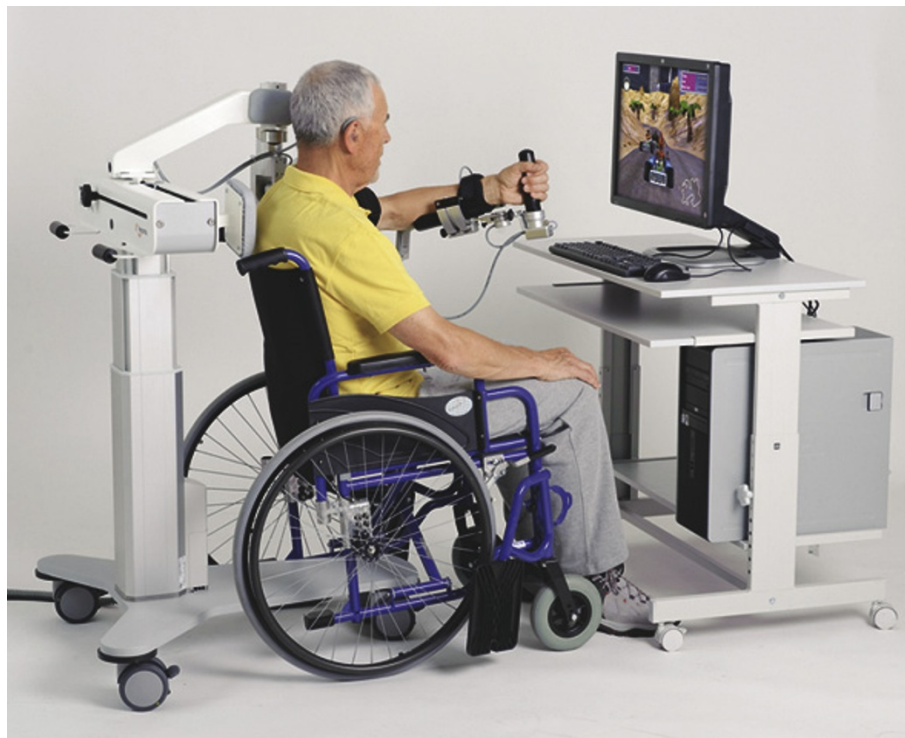
Figure 1 The experimental setup. Experimental setup using a passive device for upper-extremity rehabilitation (Armeo ® Spring, Image courtesy of Hocoma AG, Switzerland).
