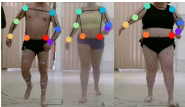
Fig. 1 Examples of labelled videos with anatomical landmarks, resulting from applying the trained networks to label videos. The anatomical landmarks identified were approximations of the shoulder, elbow and wrist centres on each arm, and the anterior superior iliac spine ridges on both sides of the pelvis. Note the physical markers that can be seen in the images were not used in this analysis
