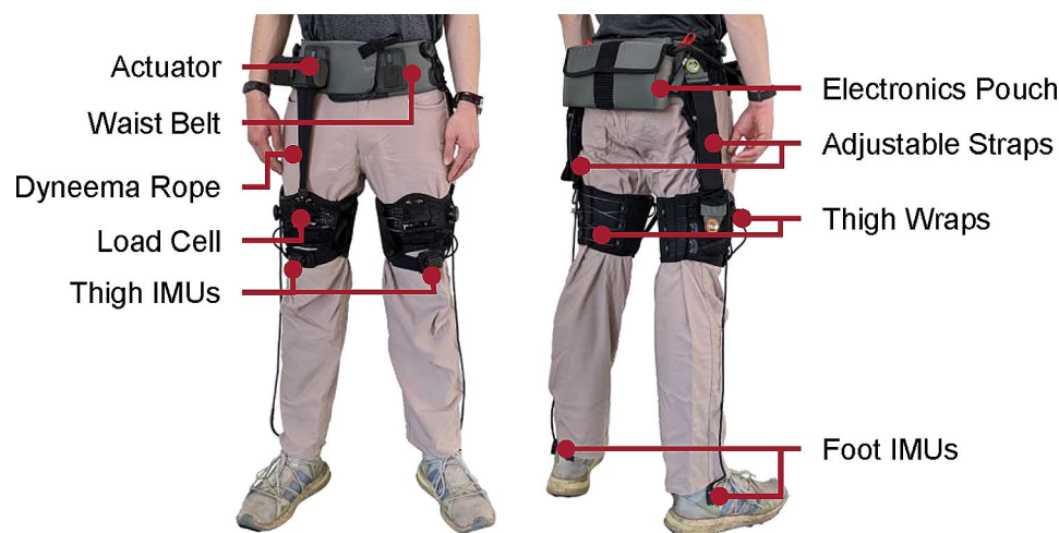
Fig. 1 Components of the unilateral hip flexion exosuit, set up for an individual with right hemiparesis. For use in individuals with left hemiparesis, the actuator and the rope would be attached to the left side
