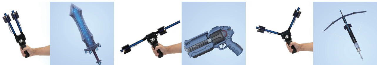
Figure 1: Transcalibur can dynamically present size of various object in VR, actuating weight and angle mechanisms. Although the actual controller's appearance differs from its appearance in VR, a user feels as if s/he is wielding a sword (left), a gun (center) and a crossbow (right) with the same VR controller.
