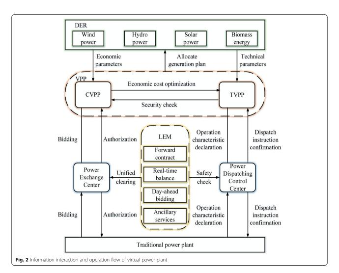
CVPP and TVPP correspond to these two characteristics respectively. Namely, to ensure the economy and security of VPP is to ensure the stable operation of CVPP and TVPP.
