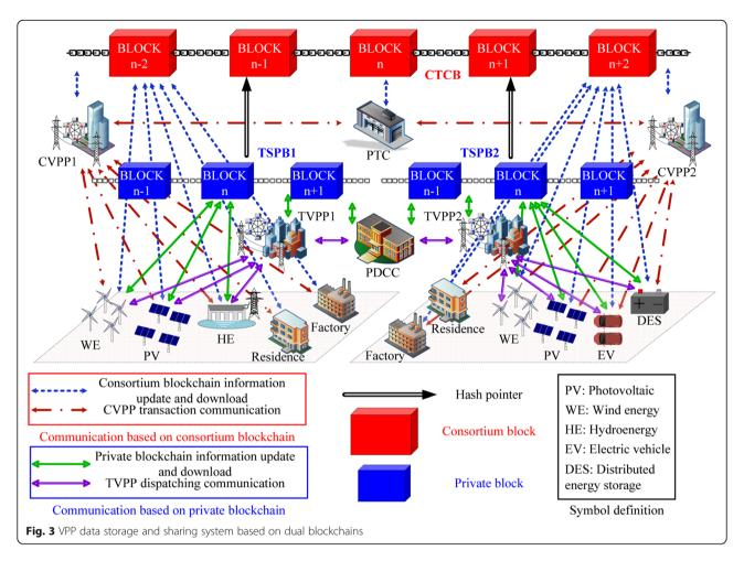
information form DER, such as energy type, working power, generation quota and other external information as for local time, geographical location, weather and so on. Using private blockchain in TVPP scheduling layer can achieve efficient, large capacity and low-cost information storage. Therefore, the purpose of this paper is to realize the complementarity of the two blockchains to form a practical information storage scheme.
