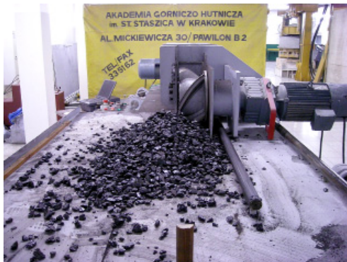
Fig. 6. Winning prism – operation without loader and k_w = 0,29
