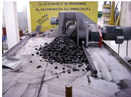
Fig. 7. Winning prism – operation without loader and k_w = 0,58
