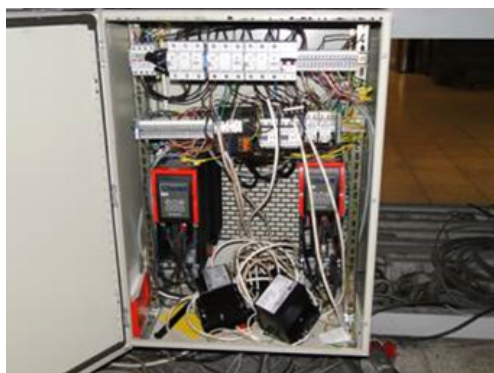
Fig. 4. Testing stand measuring system, control system cabinet at the left side and measurement computer with docking station at the right side
