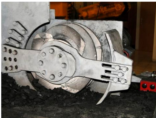
Fig. 3. Plow head equipped with curtain loader
