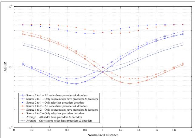
**Figure 5 ABER versus normalized distance (d).** Average BER variation with normalized distance (d) for three different design schemes. N=2,  $\gamma=4$  dB, and  $P_T/\sigma^2=32$  dB.
