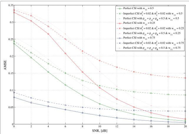
**Figure 7 AMSE versus transmit SNR: weight parameters in BC stage.** Average MSE variation for source 1 with SNR ( $\gamma$ ) for different weight parameters in broadcasting stage. N=2,  $P_T/\sigma^2=8\gamma$ .
