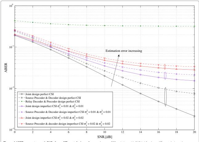
Figure 4 ABER versus transmit SNR: three different design schemes. Average BER variation with SNR ( $\gamma$ ) for three different design schemes. N = 2,  $P_T/\sigma^2 = 8\gamma$ .
