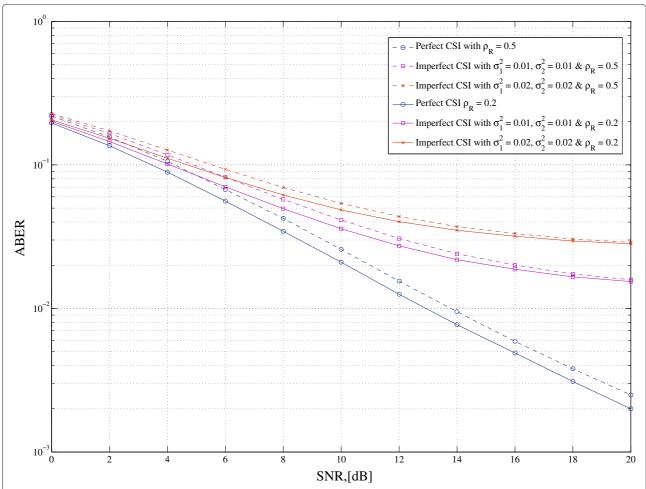
**Figure 2 ABER versus transmit SNR: relay antenna correlation and estimation error.** Average BER variation with SNR ( $\gamma$ ) for different relay antenna correlations and estimation error variances. N=2,  $P_T/\sigma^2=8\nu$ .
