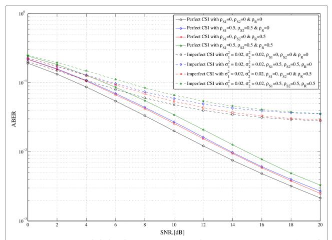
Figure 3 ABER versus transmit SNR: both relay and source antenna correlations and estimation error. Average BER variation with SNR ( $\gamma$ ) for different relay and source node antenna correlations and estimation error variances. N=2,  $P_T/\sigma^2=8\gamma$ .
