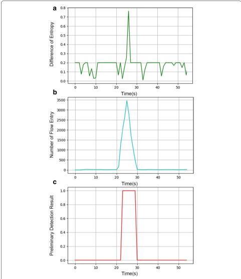
**Fig. 8** Preliminary detection result in the edge switch (SYN). **a**: Real-time results of information entropy difference. **b**: Real-time statistic results of flow entries. **c**: Detection decision in the edge switch (0 represent normal, 1 represent abnormal)
