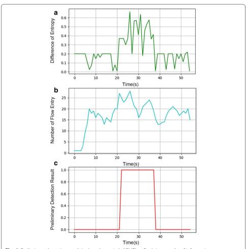
**Fig. 6** Preliminary detection result in the edge switch (ICMP). **a**: Real-time results of information entropy difference. **b**: Real-time statistic results of flow entries. **c**: Detection decision in the edge switch (0 represent normal, 1 represent abnormal)
