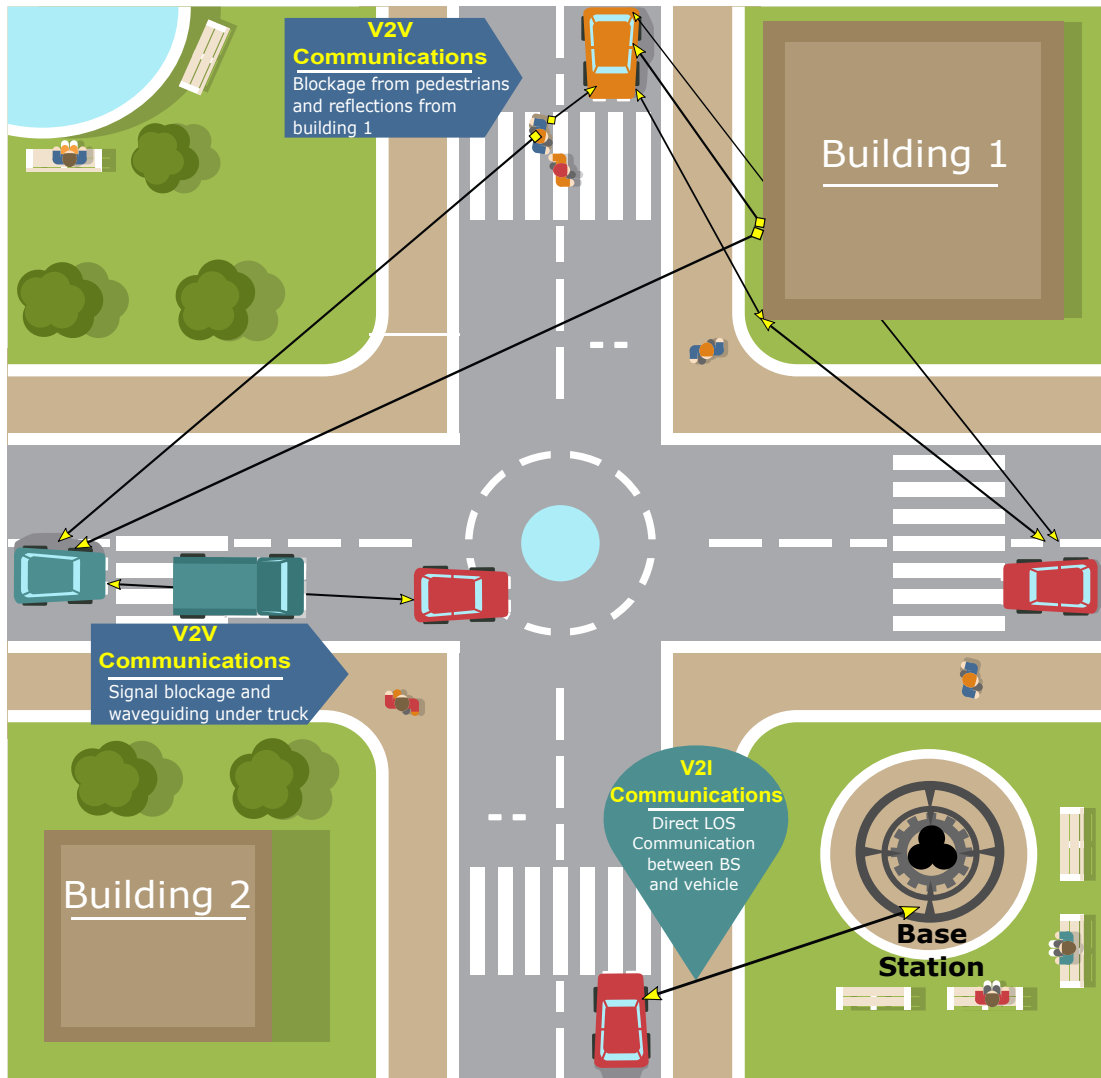
Fig. 2: Typical propagation effects and link types in mmWave vehicular communications.
