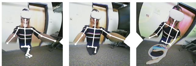
Figure 18: Pose estimation failure cases due to self-occlusion. From left to right: occlusion of lower body due to crossed legs, occlusion of feet due to kneeling and occlusion of body by the controller itself.
