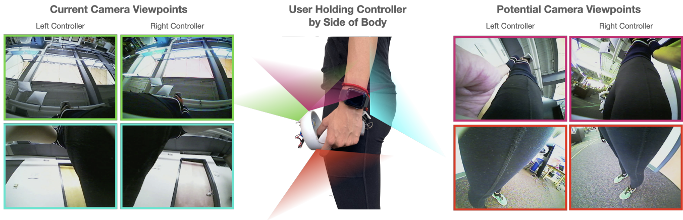
Figure 17: Example views when the controllers/hands are resting by the side of the body. Our current cameras (green & cyan) do not capture the body, and so our pipeline fails. In the future, cameras with larger fields of view could be utilized, or one or more cameras could be added to the controller. We captured examples of what these views would look like (purple & red), and it seems likely that pose models could detect the body even from this disadvantaged location in future work.
