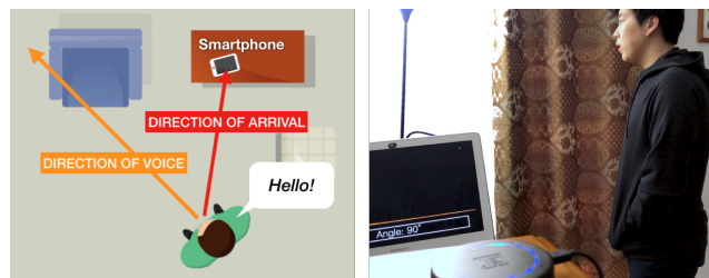
Figure 1. Left: an illustration of Direction of Voice (DoV) vs. Direction of Arrival (DoA). Right: our approach allows devices (“smartspeaker” in foreground) to compute DoV (debug output shown on laptop) without any external sensors, which could enable more robust and natural voice interactions, especially in contexts with many devices.
