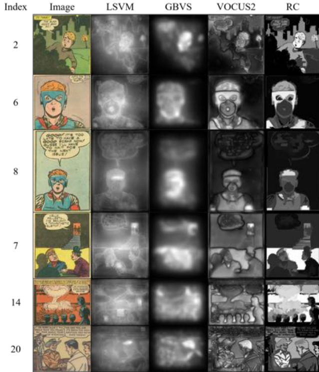
Fig. 2: Saliency maps generated from four different algorithms are depicted for chosen comic images. LSVM, GBVS show center bias, and similar regions are marked salient. VOCUS2 finds it difficult to detect multiple salient regions, whereas, RC marks complete regions as salient.
