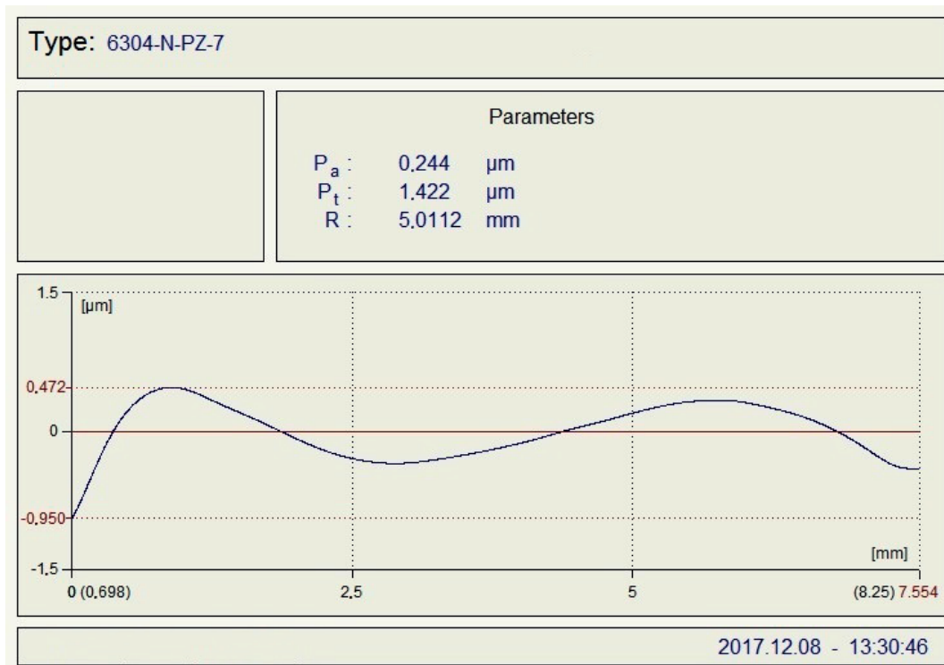
Figure 6 Outer race profile after filtration
