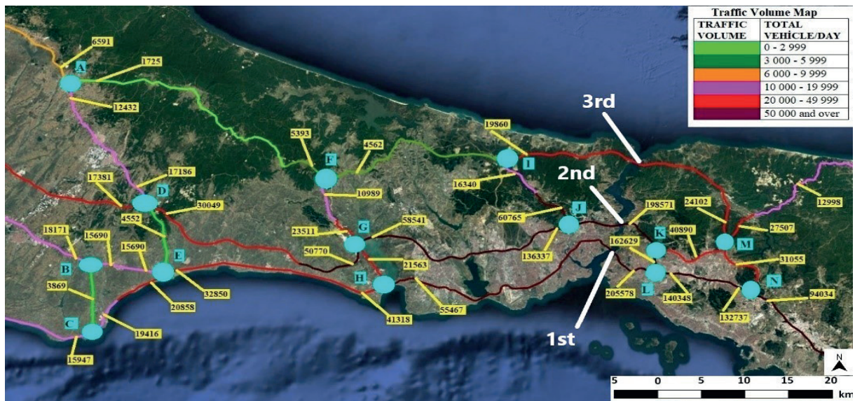
Figure 3 The second case study; traffic volume map from after the construction of the 3 rd Bosphorus Bridge and the Northern Ring Motorway (Connection of I and M intersections)
