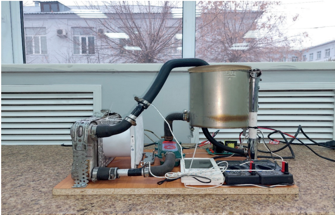
Figure 5 experimental bench for ultrasonic cleaning the car radiator
