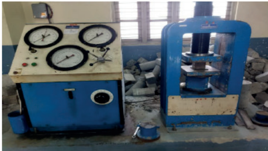
Figure 7 Compression strength test setup
