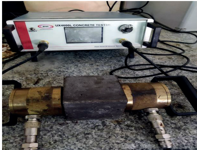
Figure 5 Ultrasonic pulse velocity test setup
