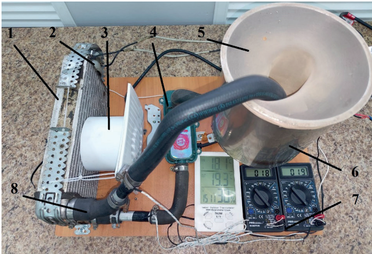
1 - interior heater radiator; 2 - ultrasonic emitter; 3 - axial fan; 4 - circulation pump with a heating element; 5 - filter; 6 - reservoir for liquid; 7 - devices for temperature control; 8 - rubber pipes
