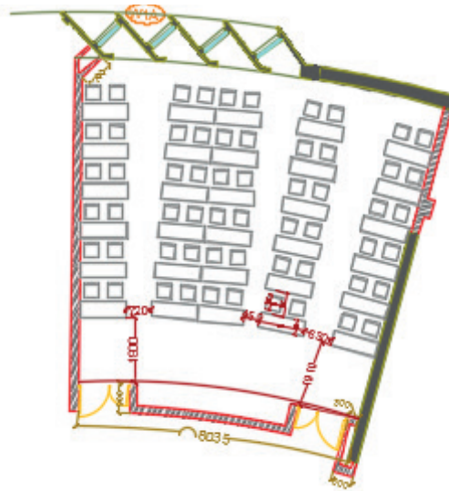
Figure 2 Sketch of a classroom experimental scenario in Lecture Hall Complex, IIT Delhi (here Corridor width 1800 mm, between benches (from left to right 720 mm, 450 mm and 630 mm respectively)
