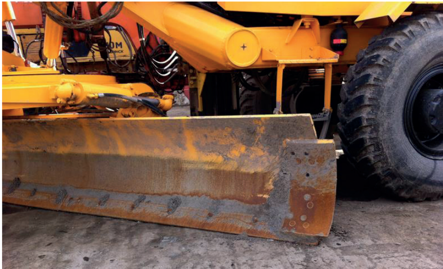
Figure 9 Wear of motor graders knives at the facilities of the trust Construction mechanization LLP
