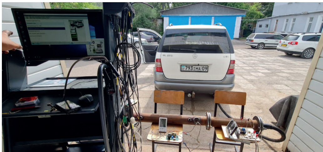
Figure 7 The process of connecting the vehicle to the diagnostic complex
