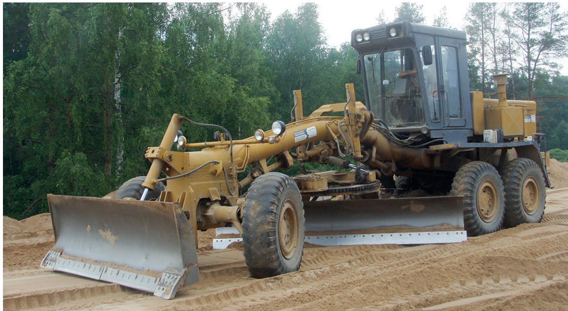
Figure 4 Investigation of the wear pattern of motor grader dumps blades in production conditions
