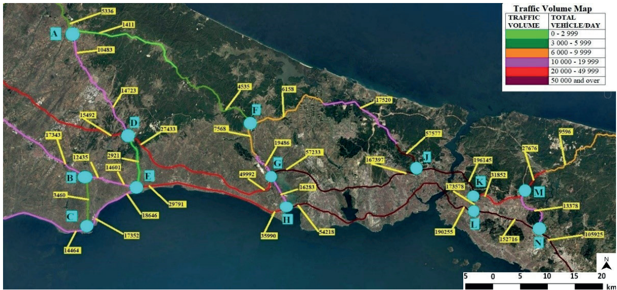
Figure 2 The first case study; traffic volume map from before the construction of the 3 rd Bosphorus Bridge and the Northern Ring Motorway
