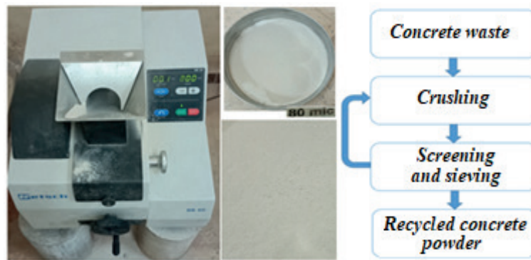
Figure 2 The manufacturing process of recycled concrete powder in the laboratory
