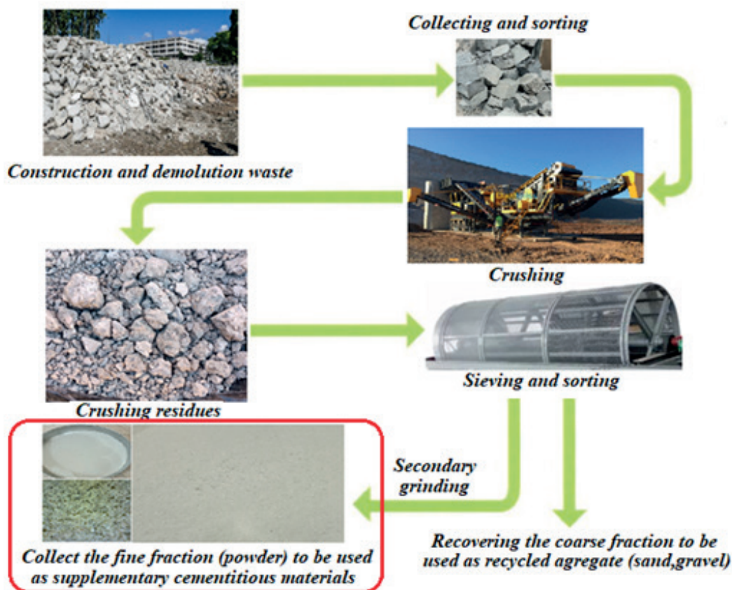
Figure 1 The concrete recycling procedure until obtaining the fine fraction
