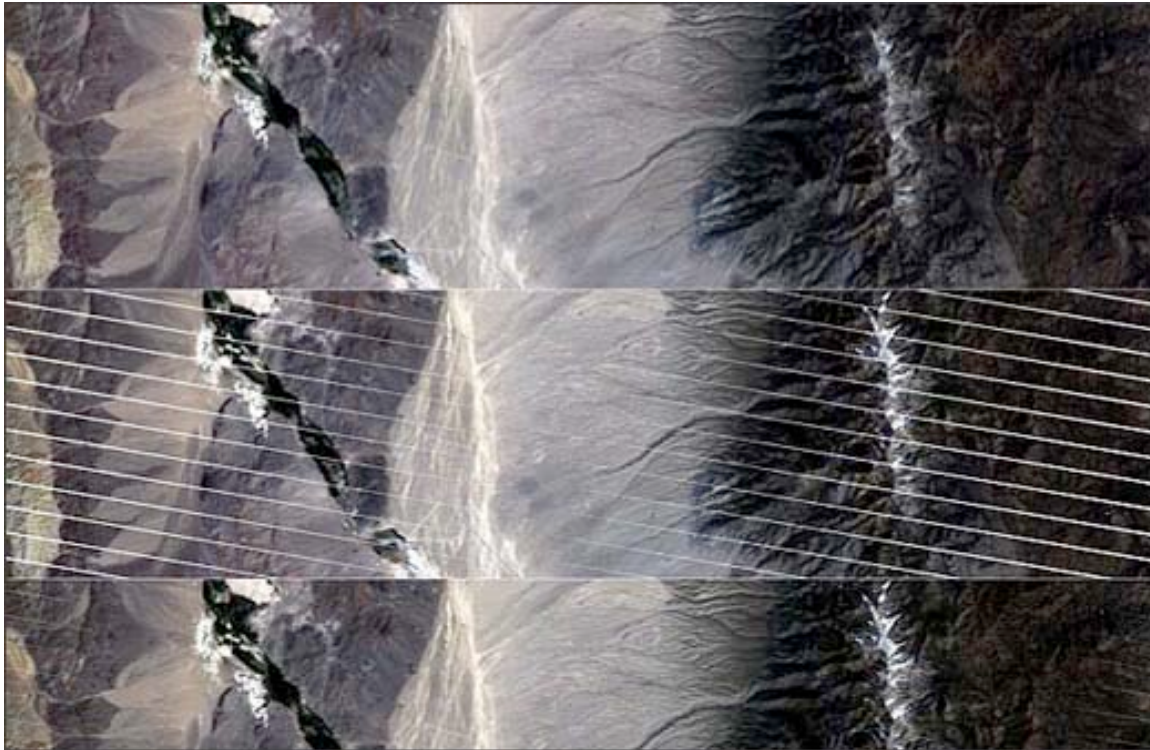
Figure 11.4 - Top image: pre-SLC anomaly, middle of image. Middle image: scene after SLC anomaly. Bottom image: scene after SLC anomaly with data gaps filled.
