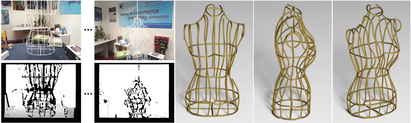
Fig. 1. We introduce CURVEFUSION, a method to reconstruct objects made of thin filament-like structures from an RGBD sequence by fusing information from noisy depth scans and loosely using RGB information for verification only.
