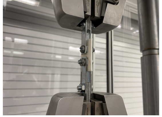
Figure 3: A 3D printed part being tested on a universal testing machine (Instron 600DX), with square nuts in the trapezoidal holes. The machine moves at a speed of 20 mm/min and stops when the object breaks or by a manual stop.
