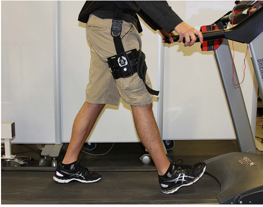
Fig. 1. Photo of human subject walking on a treadmill while wearing an IMU sensor on the thigh with a sagittal plane orientation. Thigh angle measurement follows the righthand rule.
