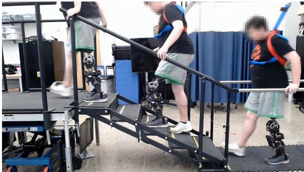
Fig. 4. Experiment setup for the controller evaluation between walking, transitions, and stair ascending. A parallel bar and a five-step staircase were placed in sequence. As a precautionary measure, the participant wore a safety harness. A licensed prosthetist fitted the powered prosthetic leg [28] to TF participants for proper alignment.
