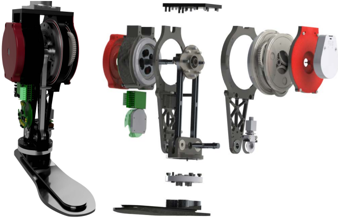
Fig. 6. CAD design of the ankle actuator. The image on the left presents the assembled ankle actuator. The exploded view on the right displays the components/sub-assemblies of the ankle actuator, such as the motor, structure, 4-bar linkage, transmission, electronics, and foot.
