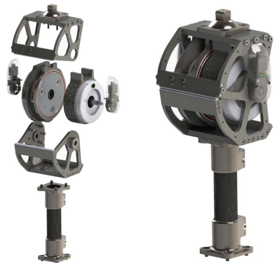
Fig. 5. CAD design of the knee actuator. The exploded view on the left displays the components/sub-assemblies of the knee actuator, such as the upper/lower hinges, encoders, transmission, motor, and pylon. The image on the right presents the assembled knee actuator. The pyramid adapter on top connects to the user's socket, and the length-adjustable pylon on bottom connects to the ankle actuator module.
