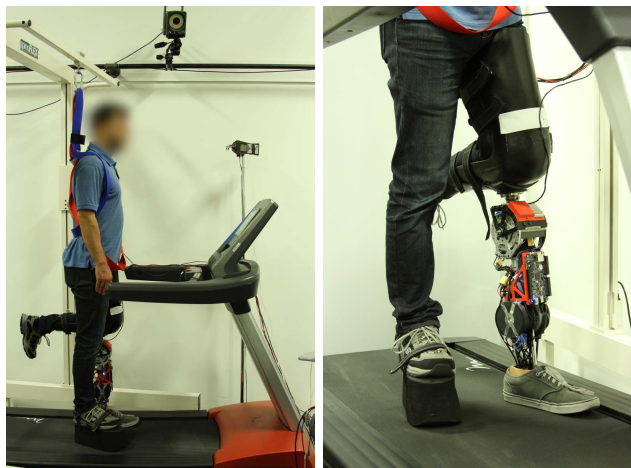
Fig. 14. Experimental setup for able-bodied walking experiments. The image on the left shows the subject, safety harness, treadmill, and sound level meter. The image on the right shows how the prosthetic leg was connected to the bypass adapter, and how it was attached to the subject's leg.
