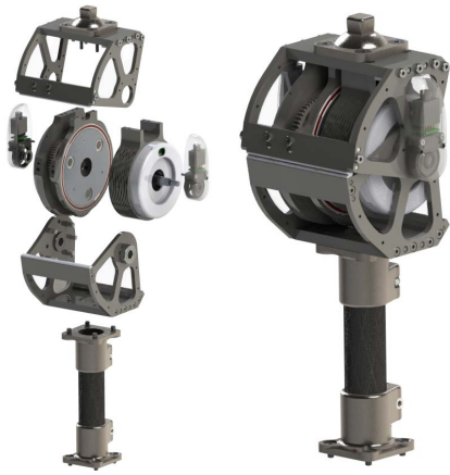
Fig. 5. CAD design of the knee actuator. The exploded view on the left displays the components/sub-assemblies of the knee actuator, such as the upper/lower hinges, encoders, transmission, motor, and pylon. The image on the right presents the assembled knee actuator. The pyramid adapter on top connects to the user's socket, and the length-adjustable pylon on bottom connects to the ankle actuator module.
