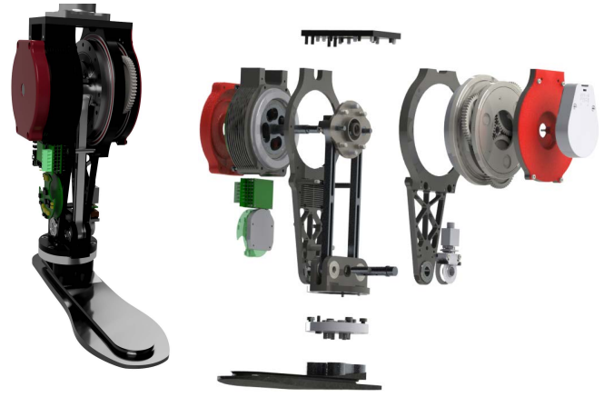
Fig. 6. CAD design of the ankle actuator. The image on the left presents the assembled ankle actuator. The exploded view on the right displays the components/sub-assemblies of the ankle actuator, such as the motor, structure, 4-bar linkage, transmission, electronics, and foot.
