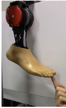
Fig. 7. Experimental setup for backdrive torque test.
