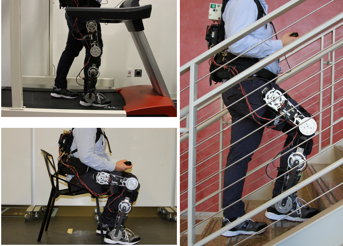
Figure 17. Photos of multiple task experiments. Top left: treadmill test, bottom left: sit-to-stand-to-sit test, right: stair ascent/descent tests.
