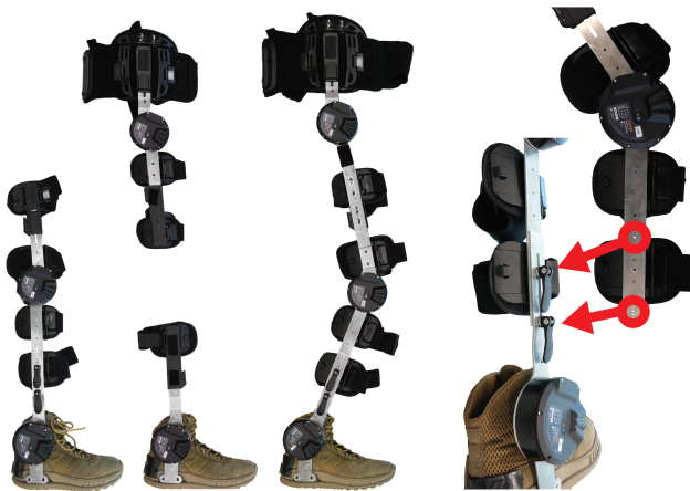
Fig. 2. M-BLUE configurations with the ankle module. The knee-ankle, hip-ankle, and hip-knee-ankle configurations are shown from left to right. The rightmost diagram illustrates the attachment of ankle and knee modules.
